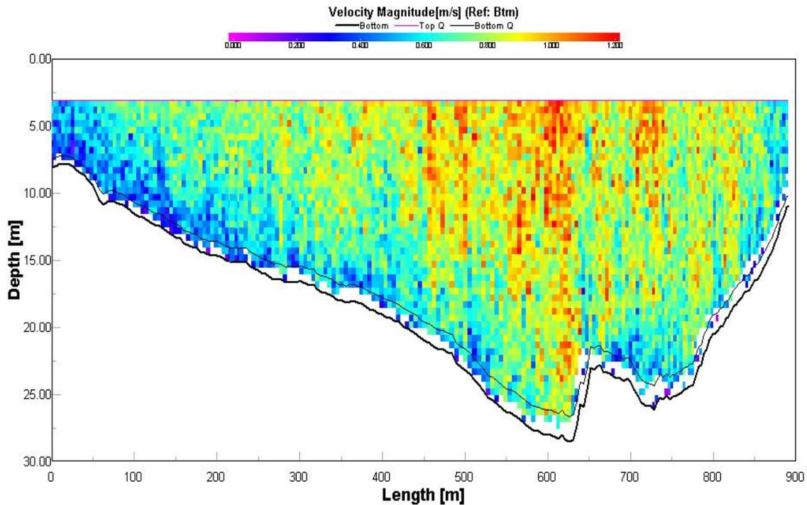
**Figure 2:** Acoustic Doppler Current Profiler cross section velocity data at site equivalent to RiverSphere (Mike Stewart, Tulane Environmental and Earth Sciences).
